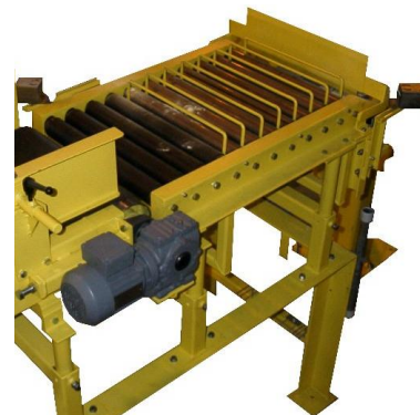
Special roller conveyor to take away sacks
