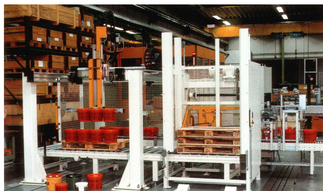
Portal-robot for palletizing buckets
